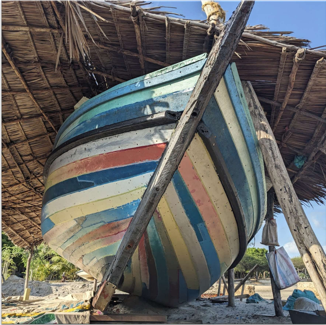
Flipflop Ndogo refitted with new bottom planking in 2024
