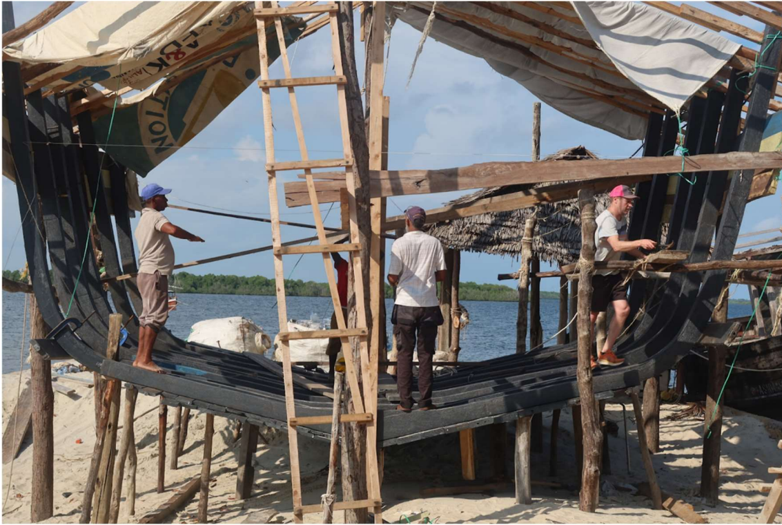
The first prototype section of Flipflop Kubwa, proving our manufacturing methods
