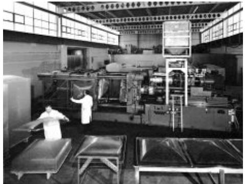
The actual injection phase — moulding 40 lbs of polypropylene from two quite different injection systems of different capacities through a Hot Runner of, an as-yet-unknown number of drops — was seen as a potential real hurdle; this, you will recall, was before MoldFlow had really taken root. Once again, fortunately, we had
