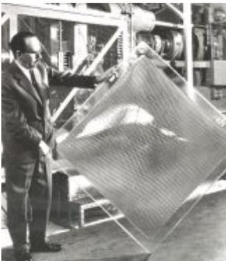
Thus, just about 0.6 T/sq.in was adequate for a 1/8th inch thick acrylic moulding with a central sprue. We now appeared to have available just marginally under 0.6T/sq.in for (probably) polypropylene (about 3/16th thick) moulded through a Hot Runner with at least three, and probably five, feeds.
