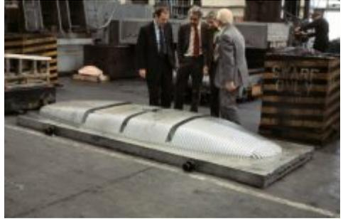
Meantime — back at the foundry — the hull presentation face has emerged before going to Shrewsbury where the first operation was to check that this hull master fitted the deck master — which it did and this confirmed that Albany had produced 2 castings, each of 8 tons and of quite different shapes, that had been cast to within 0.100 in. in 12 ft. — not at all a bad effort in precision casting!
