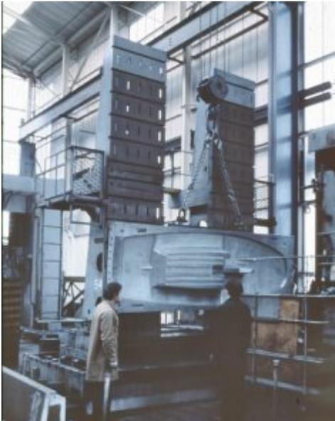
The deck casting had, by this time, arrived at Shrewsbury for machining prior to fitting into the bolster and was subject to an interested inspection by John Davies and Alan Tait who were getting their first look at an Injection Moulding tool. There was a good deal of straight machining to do and, in addition, the non presentation shut-out faces had to be profiled from the presentation face so as to produce a completely matched mould.
