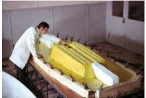
experiments and here is the deck in the clamping jig with John Hancock who master-minded this part of the operation. Expanded polystyrene blocks to aid the stability of the monocoque (and, in a crisis, buoyancy) are stuck in place, the braid is laid in the “track”, the hull component is clamped on top and two large
