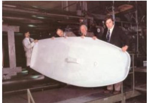
had arrived and a similar period of mould mounting and trials had taken place, a deck was moulded. This could now be mated with the hull with a water-tight joint strong enough to withstand the flexing and hammering forces imposed as Topper moved at
