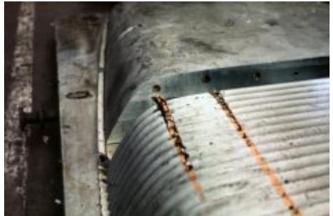
Incidentally, those deep gashes in the metal were subsequently machined out intentionally to check the depth of all the pipes in the interest of gaining maximum knowledge for future work of this sort.
