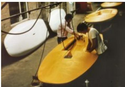
so successful, fitted out with toe-straps, dagger board housing, tiller fittings and mast lock on a production line basis, popped in Aircap and polythene sleeving.
