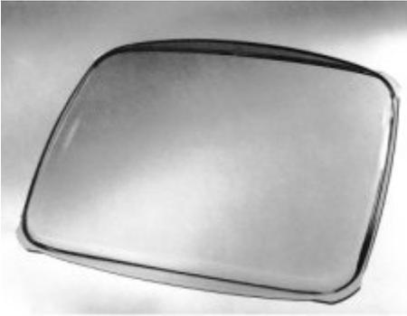
This TV screen is 450sq.in, edge-gated, about 3/16th in thick in acrylic moulded on an 800 ton press and definitely needed Injection Speed Control to keep the melt front moving at an appropriate speed.
